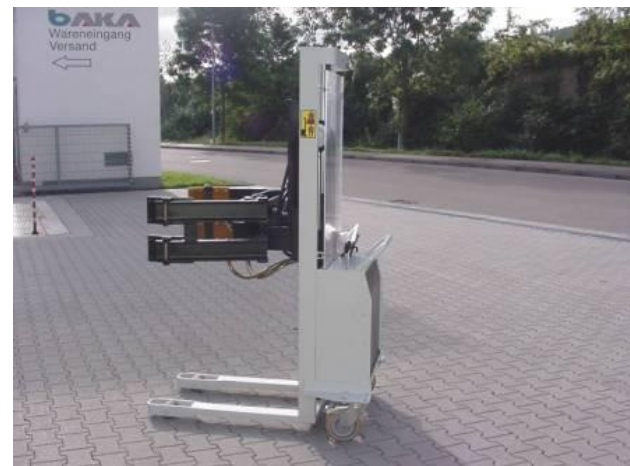
SO E 29693, E 60-604 SO, with hydraulic tensioning and rotating clamp, Load capacity 100 kg, lifting height centre clamp 280-1790 mm, Clamping range 280-520 mm
