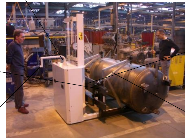
SO E 30198, E 60-1020B, Load capacity 600 kg, Lift height 1375 mm
