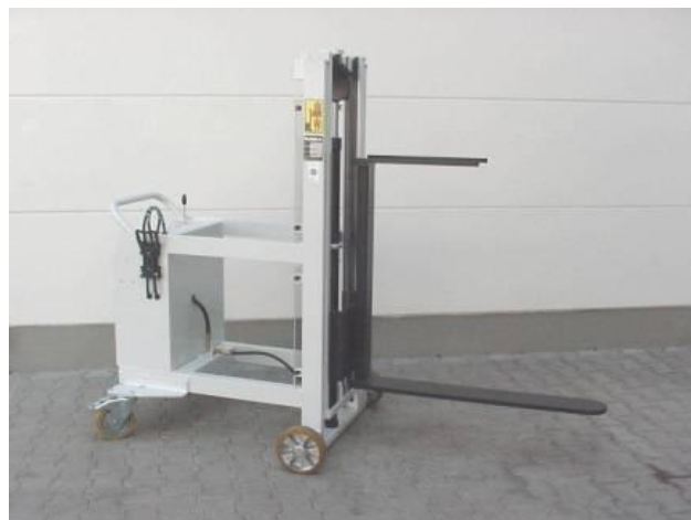
SO E 29327, E 60-SO, self-supporting with 2 side support teeth, Load capacity 100 kg, Lift height 45-2245 mm, Fork length 1000 mm
