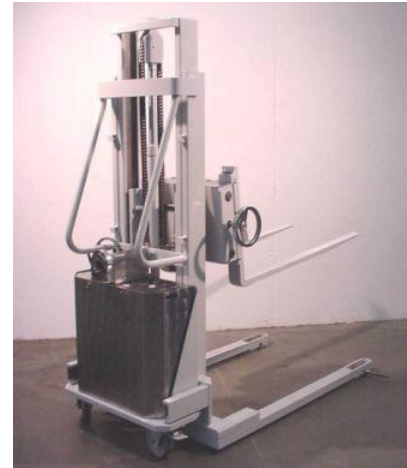
SO E 29283, Load capacity 750 kg, Lift height 50-2500 mm, hydraulic fork pitch +/- 3°, manual tooth adjustment with rod feeder
