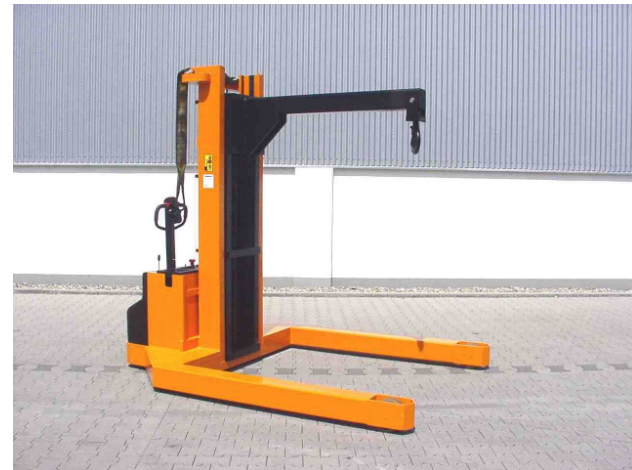
SO E 30269, EGV 2500-34, Load capacity 2500 kg at load centre distance 1400 mm, lifting height centre load hook 1800-3400 mm, broad gauge wheel arms 1920 mm
