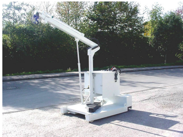
SO E 28857, EGKS 500, Load capacity 600 kg 400 kg free projection 1180 mm 2150 mm and hook height 1060-2600 mm 770-3150 mm swivel range hydraulic slide left/right 90°
