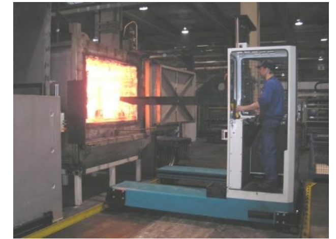
Y 316, Load capacity 1400 kg (load centre distance 1420), Lift height 3490 mm. Track-guided design for loading curing ovens
