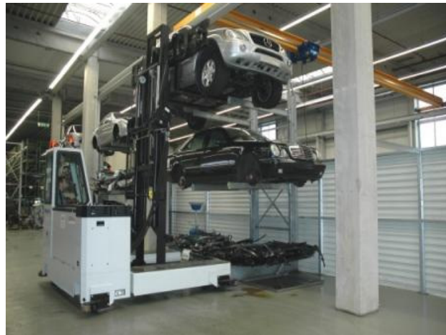
Y 279, Load capacity 3000 kg up to 6000 mm (load centre distance 800), Cabin, 3 Cameras and monitor
