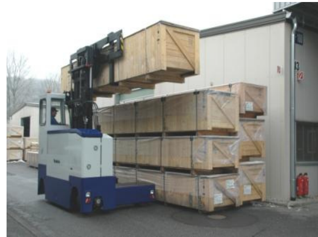
Y 317, Load capacity 7000 kg, Lift height 6000 mm, residual lifting power 6000 kg (load centre distance 600). Fork load width 500-3600 mm, hydraulic pusher forks, headlamp and rear light
