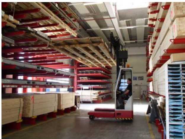
Y 293, Load capacity 3500 kg, residual lifting power 1500 kg up to Lift height 6900 mm (load centre distance 1400), Fork load width up to 2500 mm, hydraulic pusher forks
