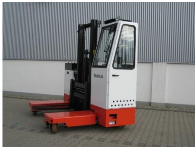
Y 320, Load capacity 2500 kg up to Lift height 4000 mm (load centre distance 550), Fork load width up to 1200 mm, hydraulic
