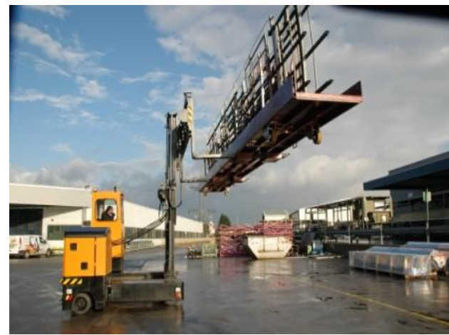
Y 319, Load capacity 4300 kg up to 3300 mm (load centre distance 2000), Fork load width 600 up to 4600 mm, hydraulic pusher forks, Heated cabin, Super-elastic-tyres
