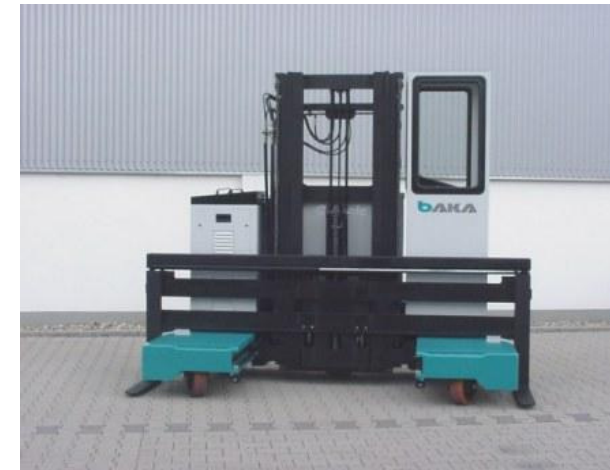
Y 302, Load capacity 2000 kg, Lift height 5500 mm, residual lifting power 800 kg (load centre distance 300), Fork load width up to 3050 mm, hydraulic
