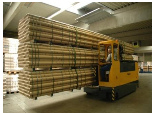
Y 322, Load capacity 8000 kg up to Lift height 3500 mm (load centre distance 600), Fork load width 500-3900 mm, hydraulic
