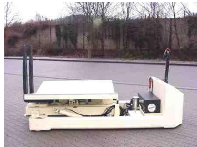
SO E 30130, with electric drawbar steering , Capacity 3500 kg, Fork length 1100 mm, additional vertical fork function , forks ca. 80-950 mm above floor, Tray rotation angle 90°
