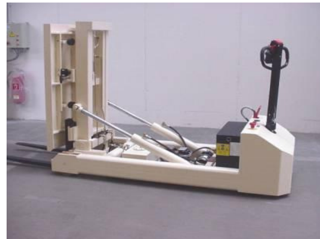
SO E 29414, Capacity 1000 kg, Fork length 1000 mm, Tray rotation angle 90° , Tray mechanically tiltable on both sides +/- 11° , Holder tray hydraulically slidable a distance of 160 mm
