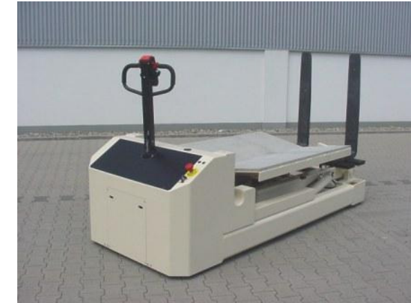
SO E 30306, with electric power steering, Capacity 3000 kg, Fork length 1100 mm, Tray rotation angle 90° , Tray manually tiltable on both sides +/- 11° , Holder tray hydraulically slidable a distance of 385 mm , Board stop manually adjustable with spindle
