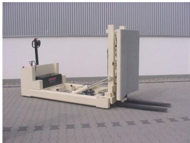
SO E 29584, Capacity 3000 kg, Fork length 1100 mm, Tray rotation angle 90° , Tray hydraulically tiltable +/- 11° , Holder tray hydraulically slidable a distance of 385 mm
