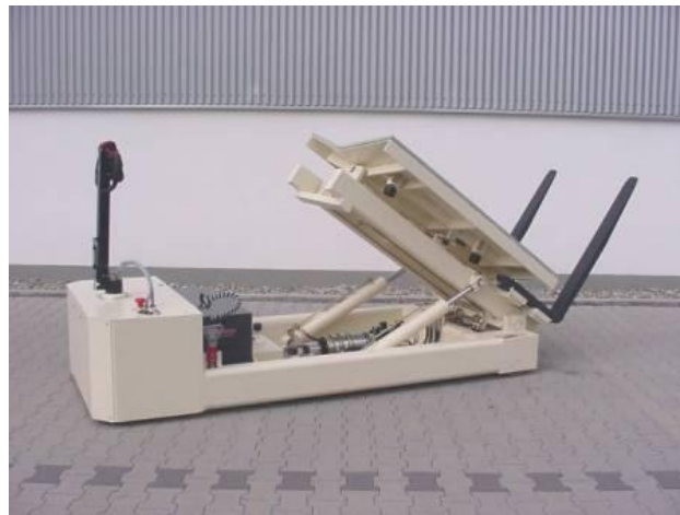
SO E 29583, Capacity 3000 kg, Fork length 1100 mm Tray rotation angle 90° , Tray mechanically tiltable on both sides +/- 11° , Holder tray hydraulically slidable a distance of 180 mm
