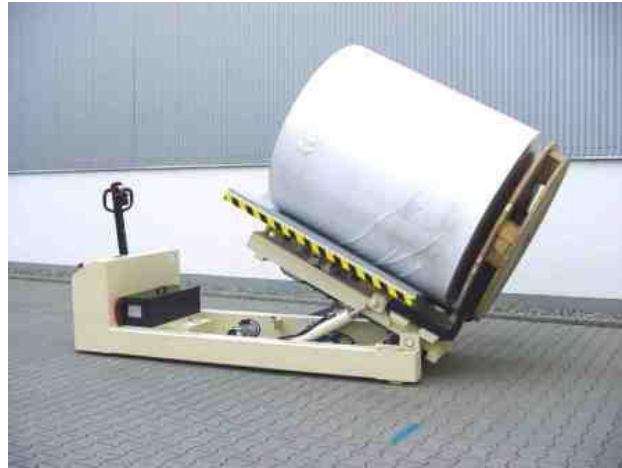
SO E 30843, with electric drawbar steering , Capacity 3000 kg, Fork length 1100 mm Tray rotation angle 90° , Tray hydraulically tiltable on both sides +/- 11°
