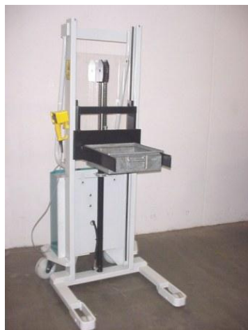
SO E 30853, E 60-1020B SO, with special load bearing capacity for customer-specific boxes 400x400 mm, Load capacity 200 kg at load centre distance 200 mm, raising/lowering with control panel (proportional hydraulics)
