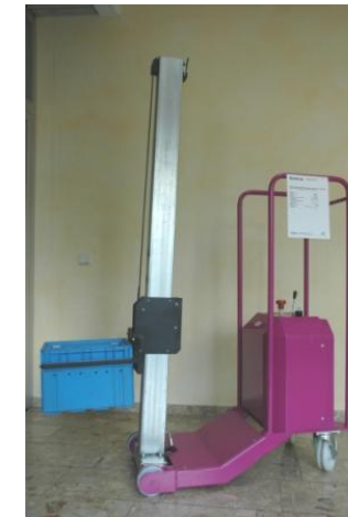
SO E 29956, E-MGS 250-15, with special forks for small load carrier container, Load capacity 250 kg at load centre distance 300 mm, Lift height 1500 mm
