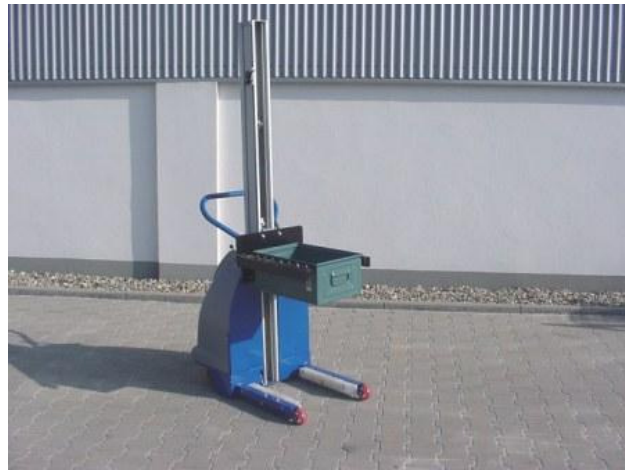
SO E 30395, ML 201 SO, Load capacity 150 kg at load centre distance 240 mm, folding forks for holding Schäfer boxes , Lift height ca. 1400 mm
