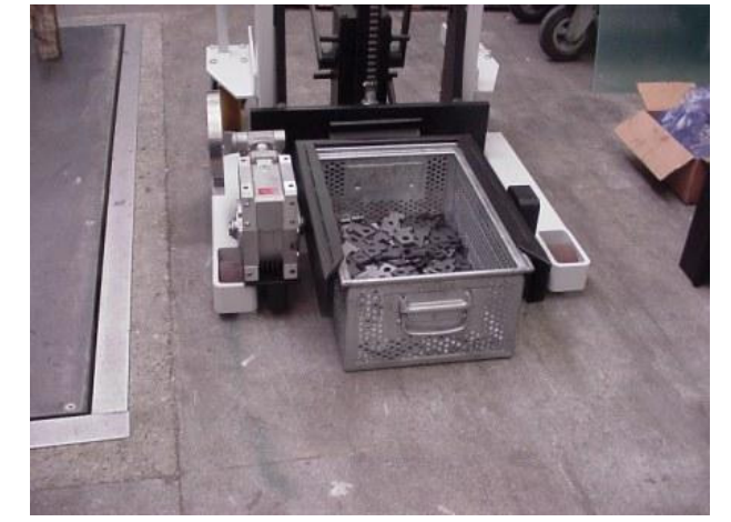
SO M 20002, HV 0,3/150, for lifting and tipping out storage boxes and cartons , Load capacity 50 kg, swivel range ca. 120°
