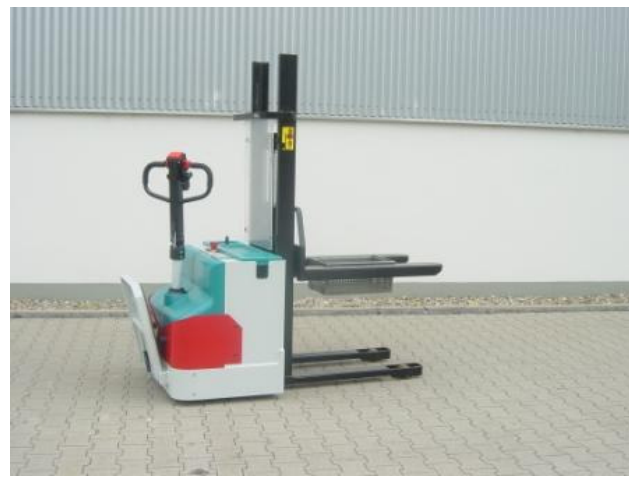
SO E 30672, EGV 1000-16 SO, for transport of Euro pallets and storage boxes , passenger standing platform collapsible, Load capacity 800 kg at load centre distance 600 mm
