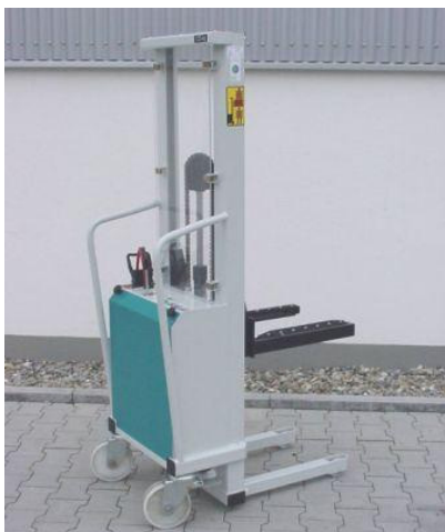
SO E 29299, E 60-SO, for holding Schäfer boxes , Load capacity 125 kg at load centre distance 250 mm, Lift height 1470 mm
