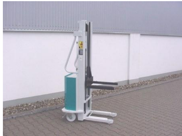
SO E 30689, ET 69-1020B, Load capacity 300 kg at load centre distance 250 mm, Lift height ca. 2100 mm, folding forks for holding storage boxes
