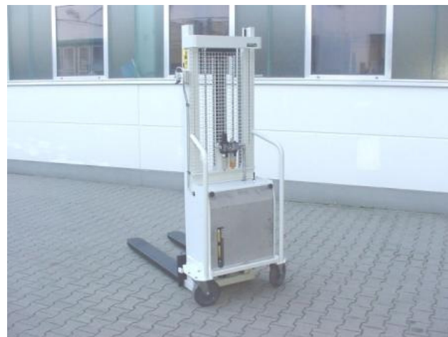
SO E 29965, Jack lift with compressed air-operated hydraulics, Load capacity 1000 kg, Lift height 2800 mm, for zone 1, cat. 2G, ex - group IIB, T3
