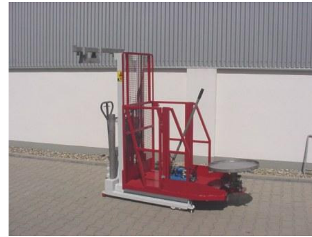
SO M 20816, Manual jack lift with work platform for zone 2, cat. 2G, ex-group IIB, T4, separate holder on the work platform for valve change, pivotable and height-adjustable
