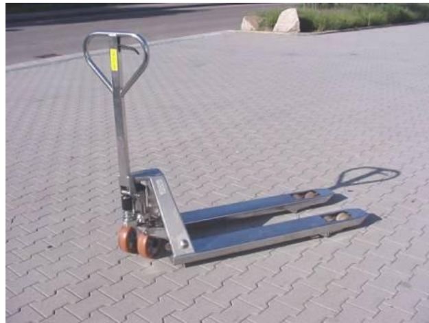
SO HU 58732-34, hand lever jack lift , Load capacity 2000 kg, Stainless steel design, for zone 1, cat. 2G, ex-group IIA, T4
