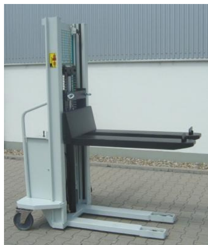
SO E 31000-01, Jack lift with compressed air-operated hydraulics, Load capacity 2000 kg, Lift height 1600 mm, transport of paint buckets ,for zone 2, cat. 2G, ex-group IIA, T3
