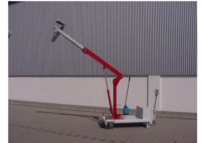
SO M 20815, Lifter with lift arm, 500 kg Load capacity at unloading 1100 mm, 280 kg Load capacity at unloading 2100 mm, for maintenance work. Swivel range ca. 22° right / left, hook height up to 2915 mm for zone 2, cat. 2G, ex-group IIB, T4
