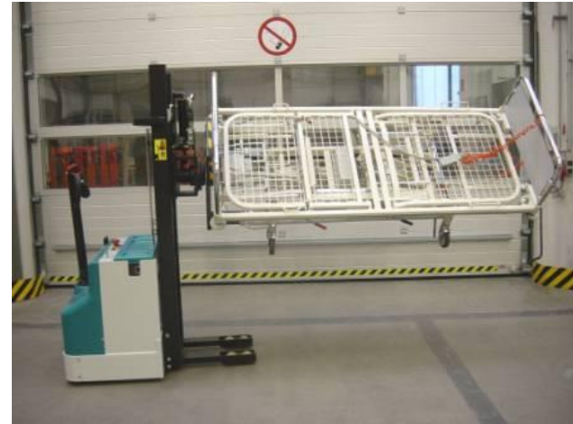
SO E 29749, EGV 1000-16, with customised holder for hospital beds, load carrier rotatable 45° left and right, Load capacity 180 kg
