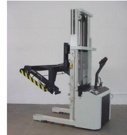
SO E 29317, EGV 4000 SO, FEM fork holder, Solid fork, fork tilt, 0-5° upwards, Load capacity 3200 kg, Lift height 190-3390 mm, Fork length 900 mm, with hydraulic tensioning for holding tools
