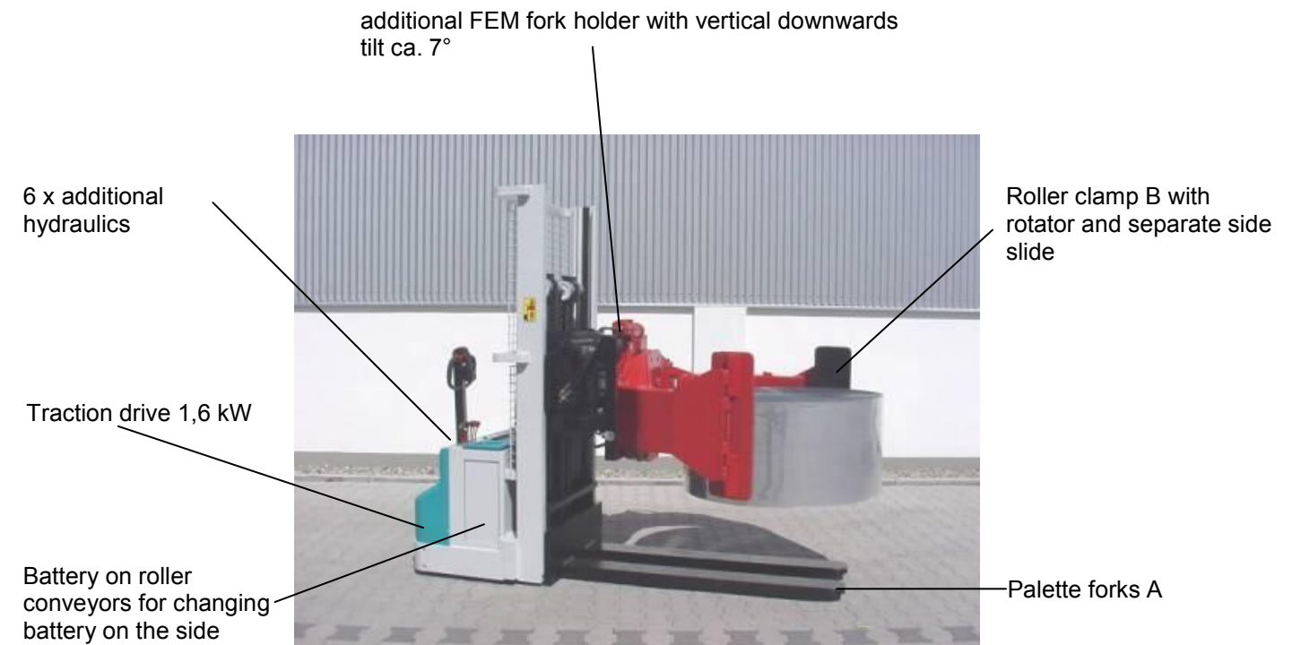
SO E 29296, EGV 2000-SO, Load capacity 1600 kg, dual lift function with 2 separate lifting sledges A Lift height fork 90-1000 mm, Fork length 1650 mm, B lifting height centre clamp 700-2000 mm, clamp opening 400-1600 mm
