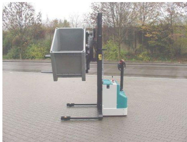
SO E 29747, EGV 1000-29, with 360° rotator, Load capacity 350 kg at load centre distance 625 mm, Lift height 50-2770 mm, solid slider fork, Fork length 1150 mm
