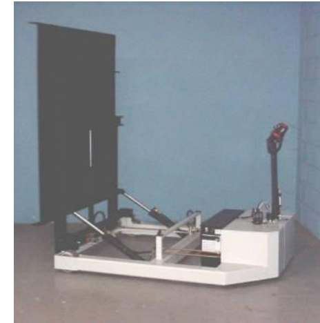
SO E 28290, EGV SO, with attached tilting and lifting platform, Load capacity 1000 kg, Platform size 1800x1600 mm, Lift height 10-410 mm, tilt angle 90°
