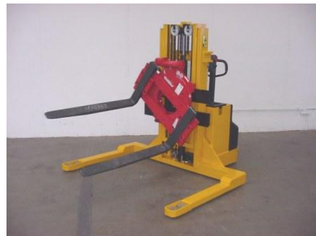
SO E 30243, EGV 2000-20, with 360° rotator Load capacity 2300 kg at load centre distance 650 mm, Lift height 2000 mm, Fork length 1200 mm
