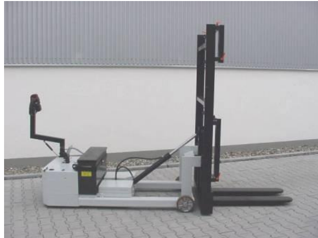
SO E 29184, EGV 1010 SO, for tilting switching cabinets, hydraulic tilting 90°, Load capacity 500 kg, Fork length 1000 mm
