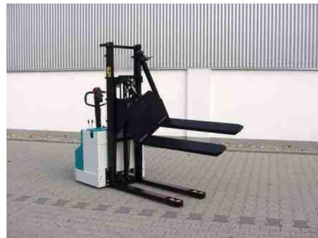
SO E 30423-24, EGV 1000-16, with lifting slides pivotable 30° on one side, Load capacity 1000 kg at load centre distance 600 mm, Lift height 90-1400 mm, Fork length 1150 mm
