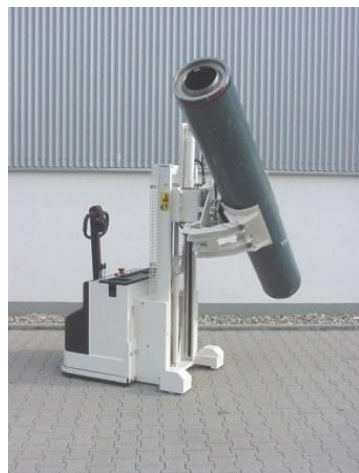
SO E 30129, EGV 0,2 SO, with attached tensioning and rotating clamp 90° rotate right, Load capacity 200 kg, lifting height centre clamping jaws 600-1500 mm, Gripper opening for Ø 356 mm
