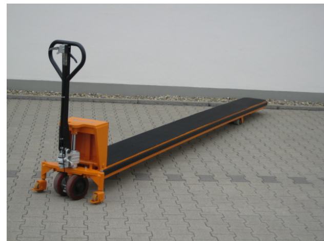
SO HU 63506, HU 2000-SO, platform jack lift, Load capacity 1500 kg, Board form length 4500 mm, Board form width 380 mm, platform with rubber support, Lift height ca. 112-217 mm, wheel brake and parking brake (drum brake), spring-born support rollers
