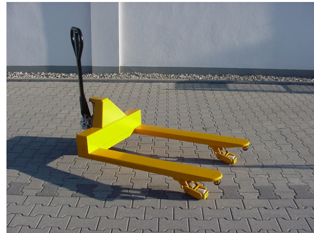
SO HU 61019, HUY 1502.2, four way jack lift, Load capacity 1500 kg, Fork length 1120 mm, Fork load width 850 mm, lifting height longitudinal movement ca. 85-165 mm, lifting height transverse movement ca. 170-220 mm
