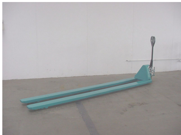
SO HU 59336, HU 3002.3 BR, Load capacity 3000 kg no load capacity reduction, Fork length 3000 mm, Fork load width 520 mm, Fork width 152 mm, Lift height 85-195 mm, with mechanical wheel brake and parking brake
