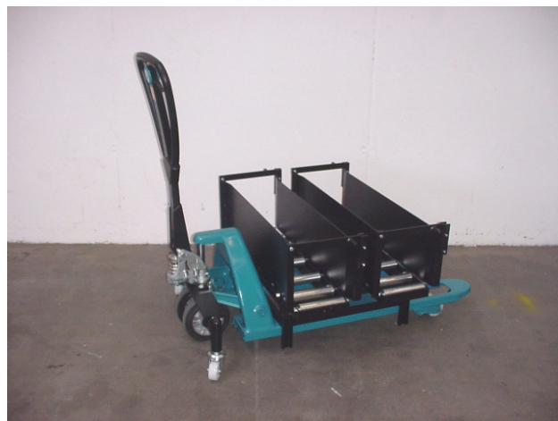
SO HU 60695, HU 2301.00-SO, battery swap lift with two attached roller conveyors, Load capacity 600 kg, Fork length 1000 mm, Fork load width 520 mm, with lateral supporting rollers
