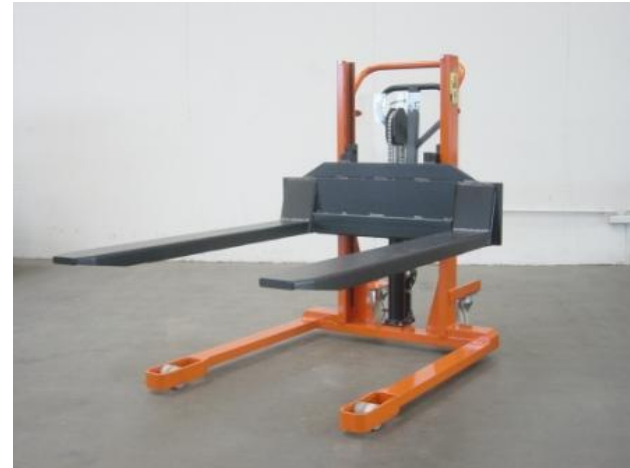
SO M 22304, M 1000-09.1, Load capacity 1000 kg at load centre distance 600 mm, Lift height 90-900 mm, Fork length 1300 mm, Fork carrying width 1000 mm
