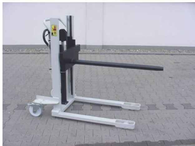
SO M 20551, M 1000-09.1, Load capacity 600 kg at load centre distance 680 mm, lifting height mandrel 120-1000 mm, suitable for paper rolls with diameter 550 mm, mandrel diameter 60 mm
