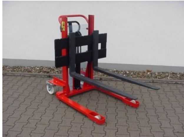
SO M 21836, M 1000-09.1 SO, Load capacity 1000 kg at load centre distance 600 mm, Lift height 60-840 mm, Fork length 1150 mm, Fork carrying width adjustable up to 900 mm, with broad gauge undercarriage
