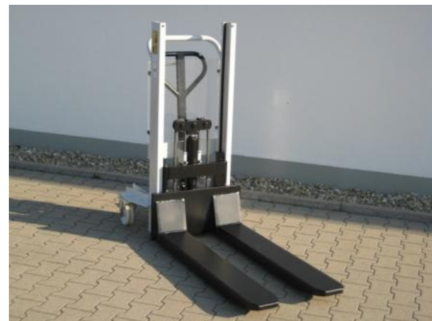
SO M 22938, M 1800-09.1, Load capacity 1800 kg at load centre distance 600 mm, Lift height 90-900 mm, Fork length 1120 mm, Fork carrying width 580 mm
