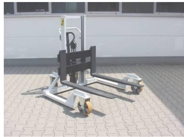
SO M 20679, M 1000-09.2 SO, Load capacity 1000 kg at load centre distance 600 mm, Lift height 45-1000 mm, Fork length 1200 mm, fork carrying width adjustable up 300-900 mm, solid slider fork
